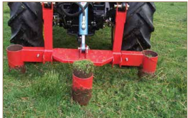
Planting can be dramatically sped up with this novel hydraulic hole-puncher which pulls PB3-sized plugs out of the ground.
