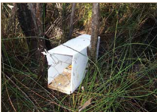
Victor professional rat trap with wire mesh to prevent accidental damage to ground foraging native birds.
