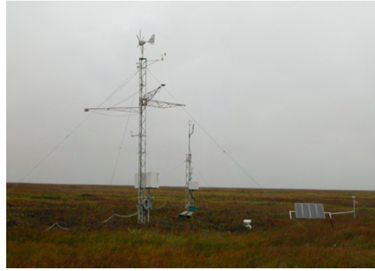
b) Installations for micrometeorological (eddy covariance) flux measurements in tundra peatlands (Indigirka lowlands, East Siberia). Photo: Andrey Sirin.
