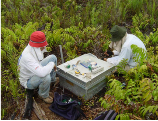
Figure 7.5: GHG flux measurements. a) Gas sampling for greenhouse gas flux determination by the closed chamber method in clear felled burned peatland at Ex-Megarice area, Central Kalimantan. Photo: Jyrki Jauhiainen.
