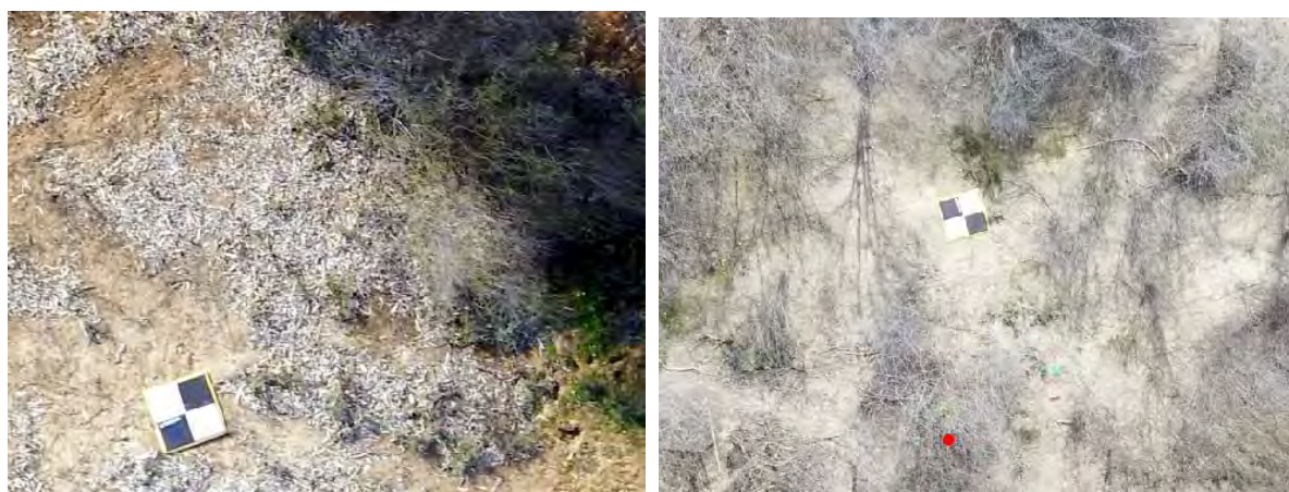
Figure 6 Sample ground control points for a) high resolution RGB imagery and b) moderate resolution RGB imagery
