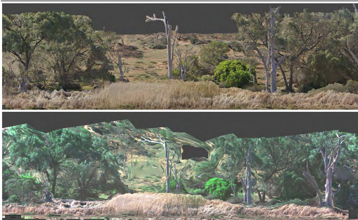
Figure 42 An area within the ortho-mosaic from the 'shallow lake' site, displaying a best-case. There are fewer artefacts in this particular section of the ortho-mosaic due to a relatively simple vegetation structure in the foreground and background. Top: RGB; Bottom: True colour multispectral composite
